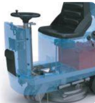
Turn on water & lower the brush head & the squeegee
