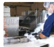
Production Conveyor Sanitising
