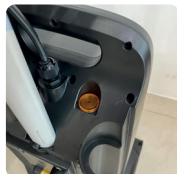
Indicator that warns if the dust bag is full or blocked
